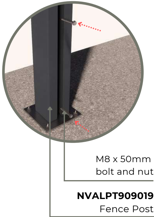
ISOMETRIC DETAIL Fence System - Model 1
